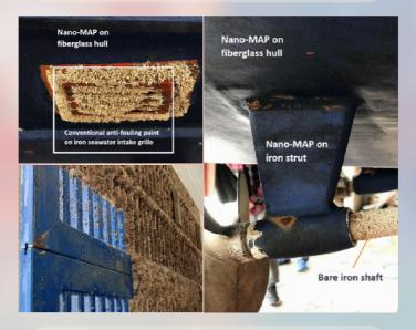
Evaluation of coating durability of the nano-photocatalytic antifouling paints on fiberglass and metal surfaces under different conditions (Fig. top left and right), including (a) single-layer painting, (b) multi-step painting techniques, (c) accelerated cycles of simulated seawater temperature variation, and (d) accelerated cycles of simulated solar radiation variation.
